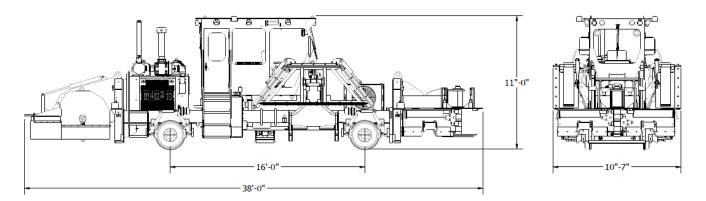
Knox Kershaw's KBR925 Ballast Regulator is a powerful track dressing machine. It comes equipped with a one pass type plow, reversible side wings, and a broom attachment. The machine features a rear mounted engine and a spacious, high visibility cab with unique window placement and hydraulic tilting function. Machine meets or exceeds all FRA requirements. Machine is customizable for converting to multiple gauges ranging from 1435 mm (56.5") to 1676 mm (66").
