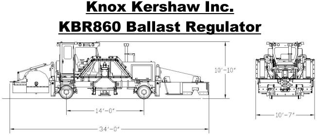
Knox Kershaw's KBR860 Ballast Regulator is a powerful track dressing machine. It comes equipped with a one pass type plow, reversible side wings, and a broom attachment. The machine features a sturdy, high visibility cab with unique window placement. The overall length and height is short to facilitate transport to the work site. Machine meets or exceeds all FRA requirements.
