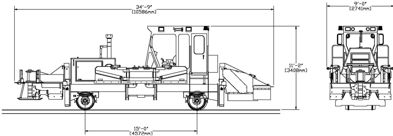
Knox Kershaw's KNG800 Narrow Gauge Ballast Regulator is a powerful track dressing machine. It can be equipped with a one pass type plow, reversible side wings, and a broom attachment. The machine is built on a mainframe which allows easy access to components. The machine is offered with an optional kit for conversion to other rail gauges.
