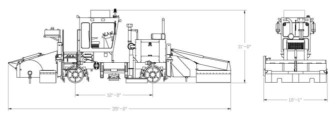
Knox Kershaw's KDB600 Double Broom is designed for sweeping excess ballast from track. With this dual broom action, the track is cleared in a single pass. The side mounted ridge plows plow down any windrow left by the front broom.
